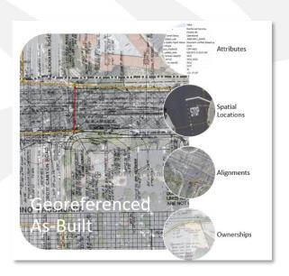
The spatially rectified facilities will be used in conjunction with the georeferenced as-builts to readjust storm drain alignments, and to identify other paved-over facilities, such as junction boxes and transition structures. The georeferenced as-builts will also be used to record storm drain materials, diameter/dimensions, lengths, and upstream and downstream inverts (both original and converted NAVD88 datum).
