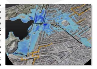
The City's drainage facilities to the east are subjected to high velocities because of the steep terrain. Wood Rodgers will model appropriate junction bend losses to reflect the hydraulic performance and deficiency of the steep storm drains which are often overlooked in simplified models. Entrance and exit losses are also crucial within the interaction of storm drains, culverts, and open channels, and will be modeled to accurately account for the hydraulic performance.
